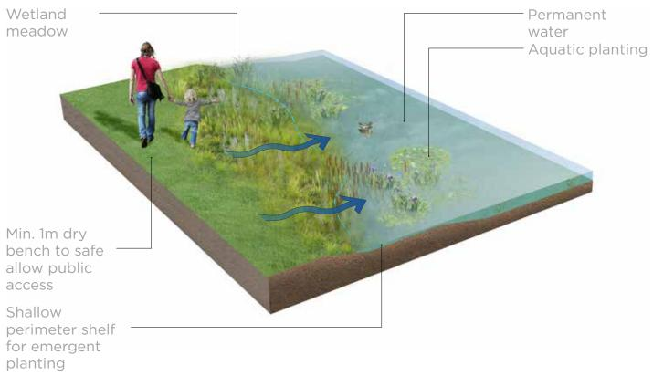
Figure 6.40 Wetlands Axonometric View
