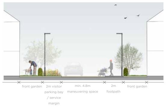
Figure 6.19 Typical Local street section
