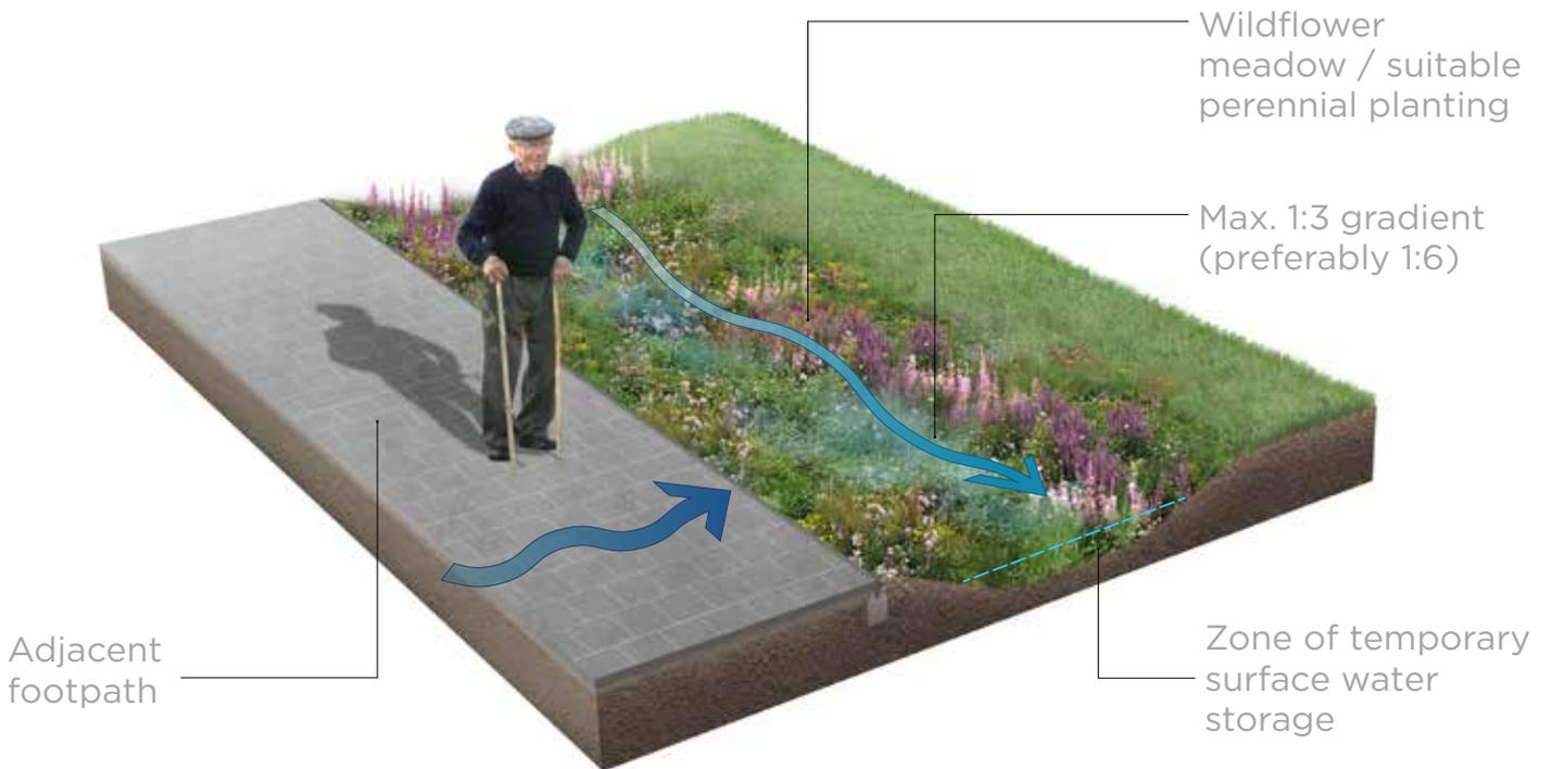
Figure 6.41 Swale Axonometric View
