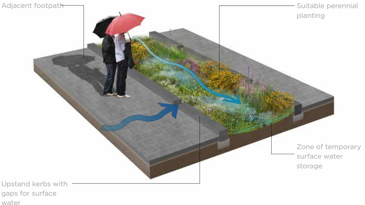
Figure 6.42 Rain Garden Axonometric View
